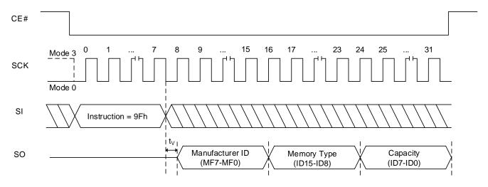
Figure 8.53 RDJDID and RDJDIDQ (Read JEDEC ID) Sequence In QPI Mode
