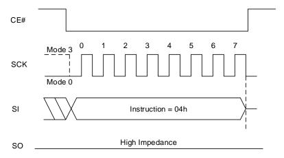
Figure 8.25 Write Disable Sequence In QPI Mode
