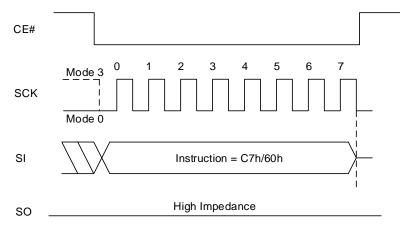
Figure 8.21 Chip Erase Sequence In QPI Mode
