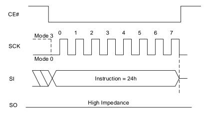
Figure 8.73 Sector Lock Sequence In QPI Mode
