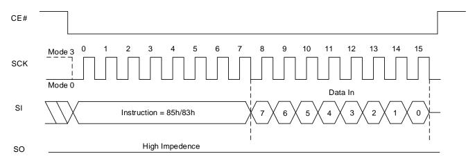
Figure 8.43 Set Extended Read Parameters Sequence In QPI Mode
