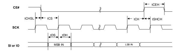
Figure 9.3 SERIAL INPUT TIMING (DTR Mode)
