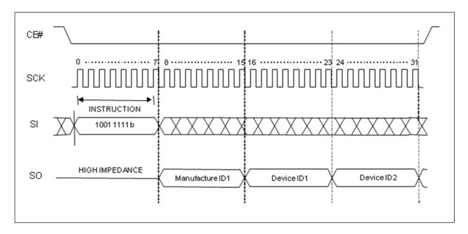
Figure 6. Read Product Identification by JEDEC ID READ Sequence
