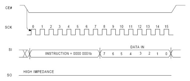
Figure 11. Write Status Register Sequence
