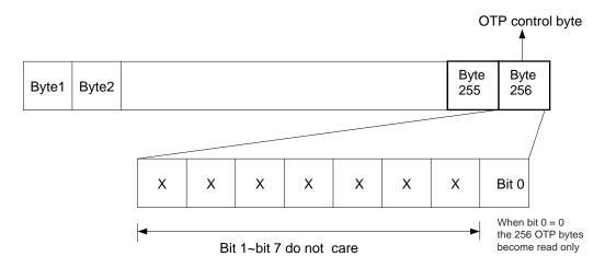
Figure 27. Control Byte to lock security memory
