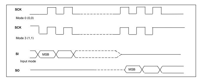
Figure 4. SPI Mode 0 and 3
