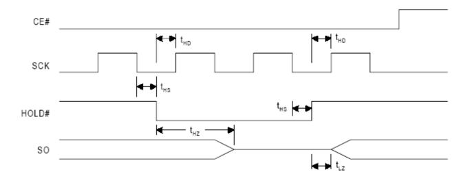
Figure 2. HOLD Timing Diagram
