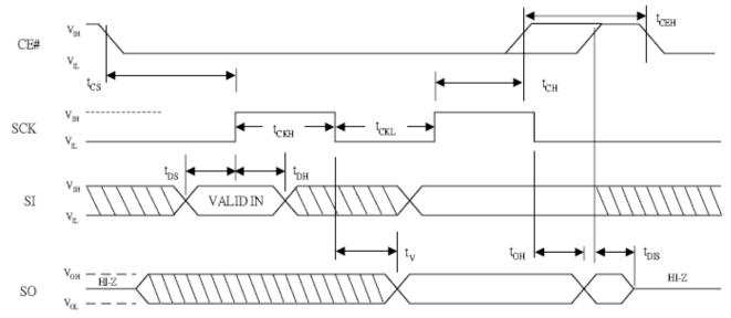
Figure 31. SERIAL INPUT/OUTPUT TIMING (1)
