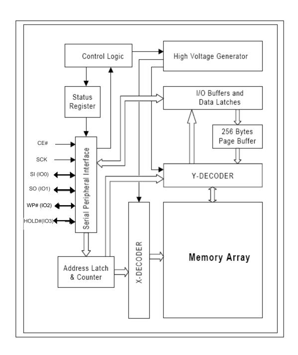
Figure 1. Flash Block Diagram
