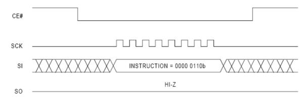
Figure 8. Write Enable Sequence
