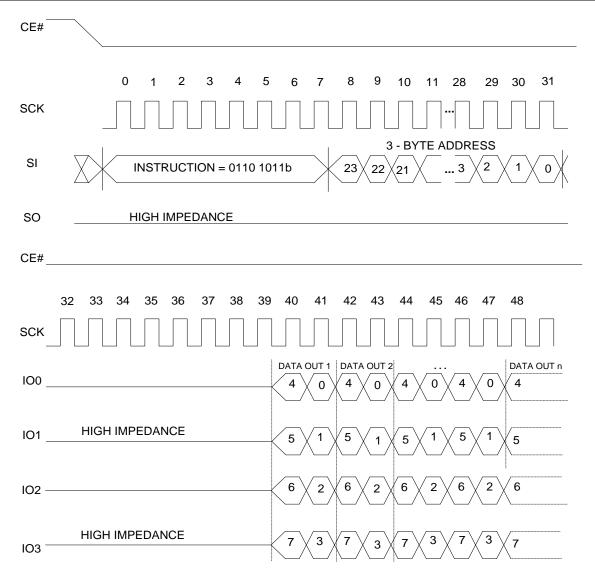
Figure 17. Fast Read Quad-Output Sequence
