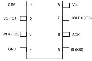
8-pin SOIC 208mil (Package: JB) 8-pin SOIC 150mil (Package: JN) 8-pin VVSOP 150mil (Package: JV)
