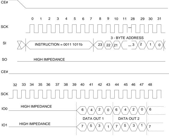
Figure 14. Fast Read Dual-Output Sequence
