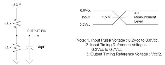
Figure 33. Output load test and input test waveform and measurement levels
