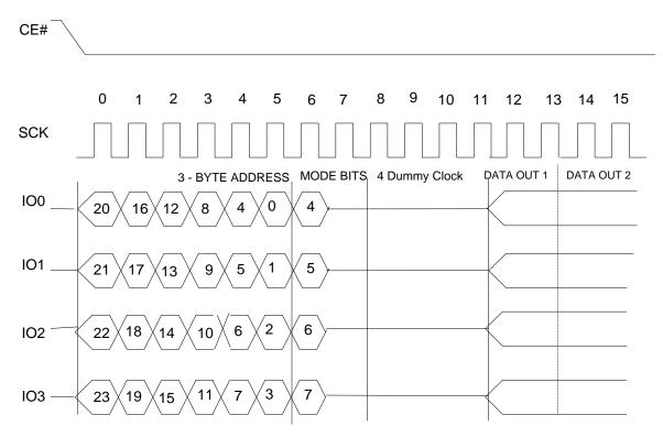
Figure 19. Fast Read Quad I/O Sequence (without command decode cycles)
