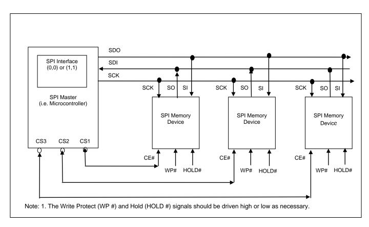
Figure 3. Conceptual Diagram using an SPI Master with Multiple SPI Flash Memory Devices
