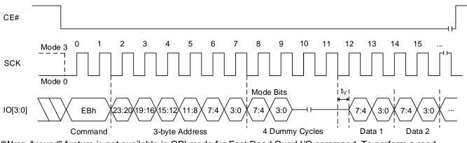
"Wrap Around" feature is not available in QPI mode for Fast Read Quad I/O command. To perform a read operation with fixed data length wrap around in QPI mode, a dedicated "Burst Read with Wrap" (0Ch) command must be used.
