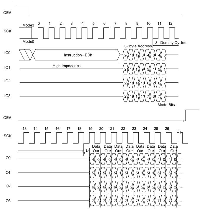
Figure 8.59 FRQDTR Sequence (with command decode cycles)
