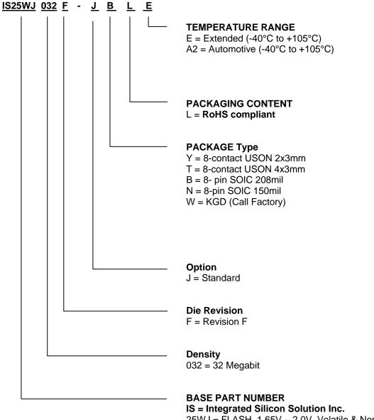
25WJ =  $\overline{F}LASH$ , 1.65V ~ 2.0V, Volatile & Non-Volatile Status Register
