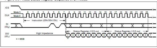
Figure 8.31 Read Status Register Sequence In SPI Mode
