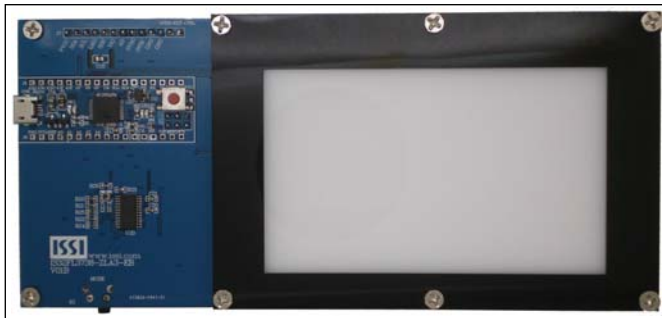
Figure 1: Photo of IS32FL3738 Evaluation Board
