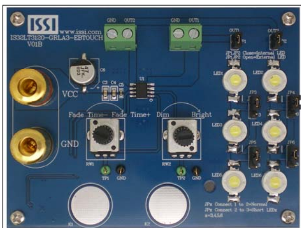
Figure 1: Photo of IS32LT3120+IS31SE5100 Evaluation Board
