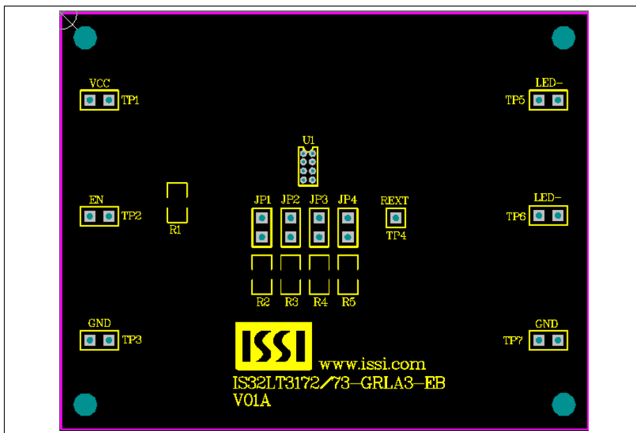
Figure 3: Board Component Placement Guide - Top Layer
