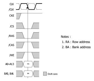
Once a row is Open(with an ACTIVE command) a READ or WRITE command may be issued to that row, subject to the tRCD specification. tRCD(min) should be divided by the clock period and rounded up to the next whole number to determine the earliest clock edge after the ACTIVE command on which a READ or WRITE command can be entered.
