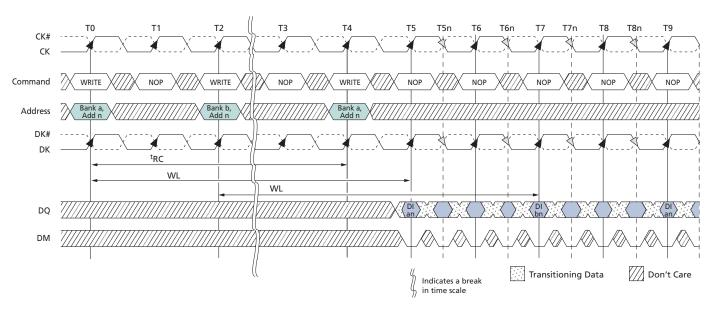
Note: 1. DI an (or bn or cn) = data-in for bank a (or b or c) and address n.
