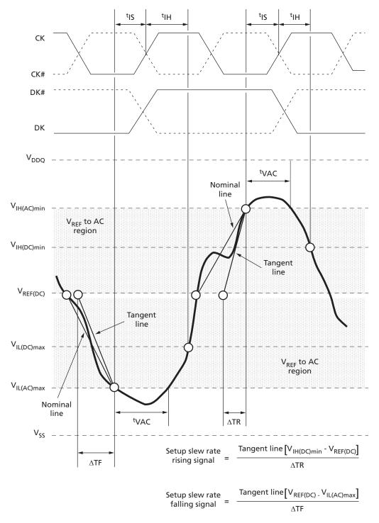
Note: 1. Both the clock and the data strobe are drawn on different time scales.
