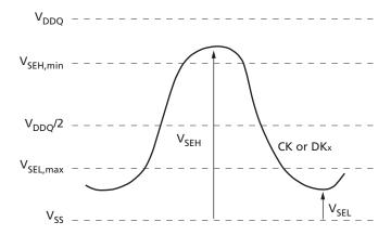
Figure 10: Definition of Differential AC Swing and <sup>t</sup>DVAC
