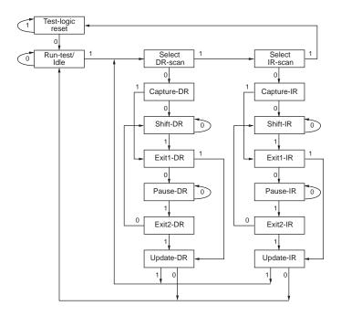
Figure 71: TAP Controller Functional Block Diagram
