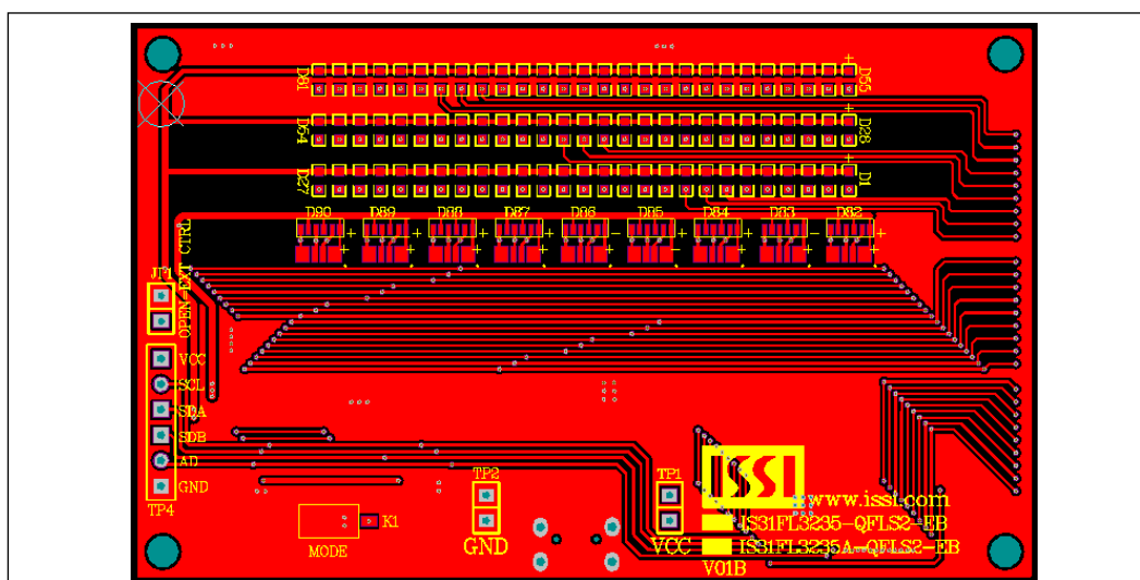
Figure 5: Board PCB Layout - Top Layer
