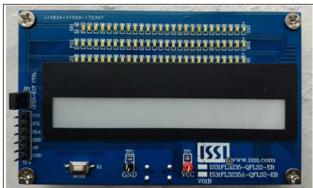
Figure 1: Photo of IS31FL3235/IS31FL3235A Evaluation Board
