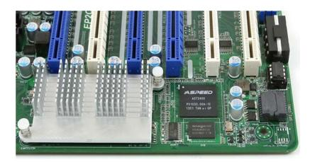
The newest AST2500 series controller from ASPEED (shown below) is used in servers from all major OEMs to hyper-scale switches in the datacenters.
