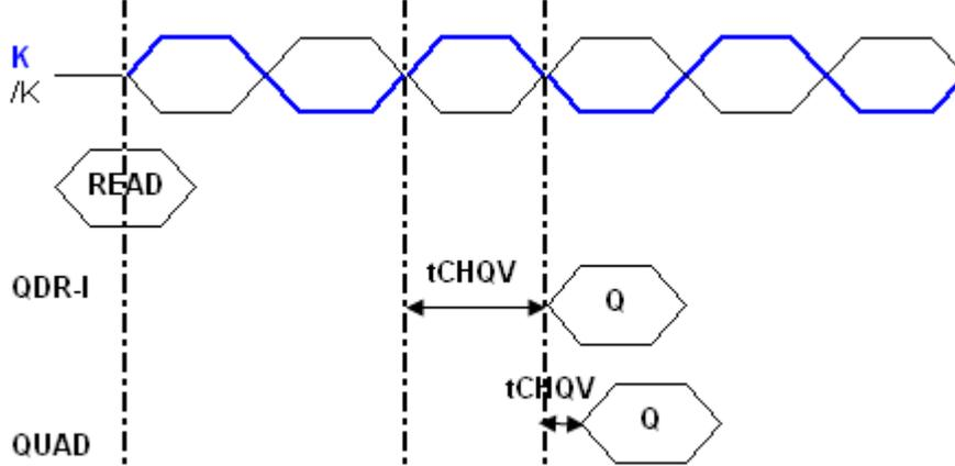
The DLL locks to the input clocks. It requires a stable C, /C or K, /K input for a minimum  $t_{KC-lock}$  ( $=1024$  cycle) period. When it is locked, the input clocks must have a low phase jitter, which is specified at  $t_{KC-VAR}$  in the datasheet. If the input clocks have jitter of more than  $t_{KC-VAR}$ , the DLL must execute the DLL reset procedure.
