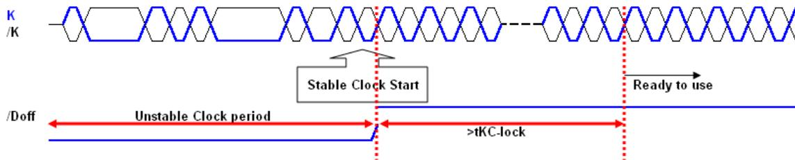
If  $\text{/Doff}$  needs to be high during power up, then  $\text{/Doff}$  must be low for a period of at least  $t_{\text{DoffLowToReset}}$  period and then return to a high level for the DLL to reset to the stable clock.
